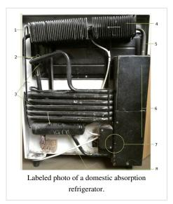
bottom of an uphill series of tubes, into which water is added at the top. The ammonia dissolves in the water, producing a mixture of ammonia solution and hydrogen. The hydrogen is collected at the top of the absorber, with the ammonia solution collected at the bottom.
